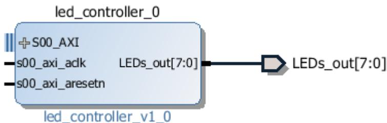
**Figure 4.10:** led\_controller block with external port
