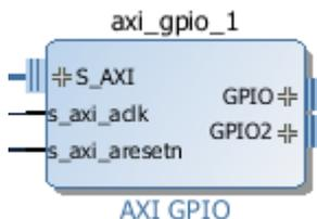
**Run Connection Automation** for **/axi\_gpio\_1/GPIO** and select **btns\_4bits** as the option for **Select Board Interface**.
